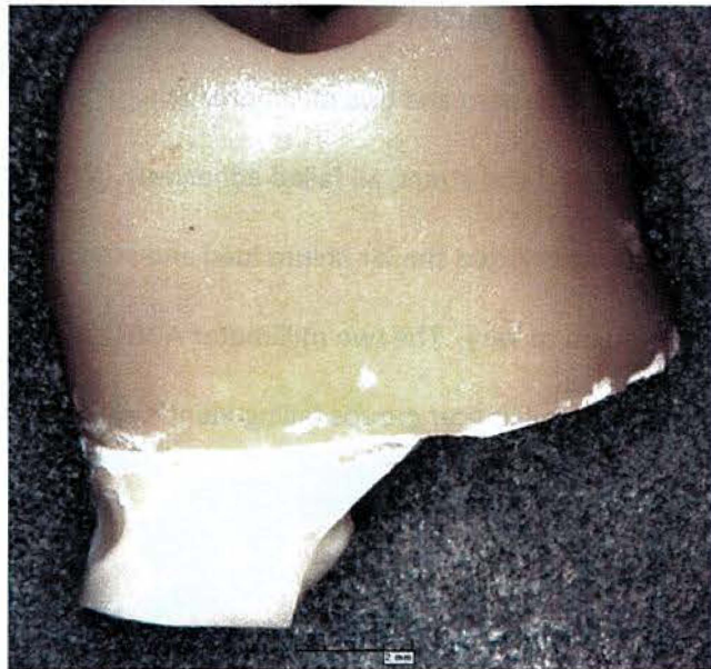
Figure 9. 20x Microscopic image of Catastrophic Failure in a Three Millimeter Sample
