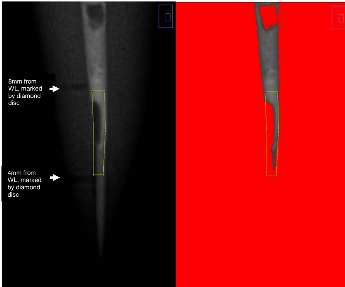
Figure 3 – Identifying void space in sample radiograph using ImageJ software. By adjusting optical threshold value, the area of voids (low radiopacity) can be measured in the confined area of interest (4mm – 8mm from WL).
