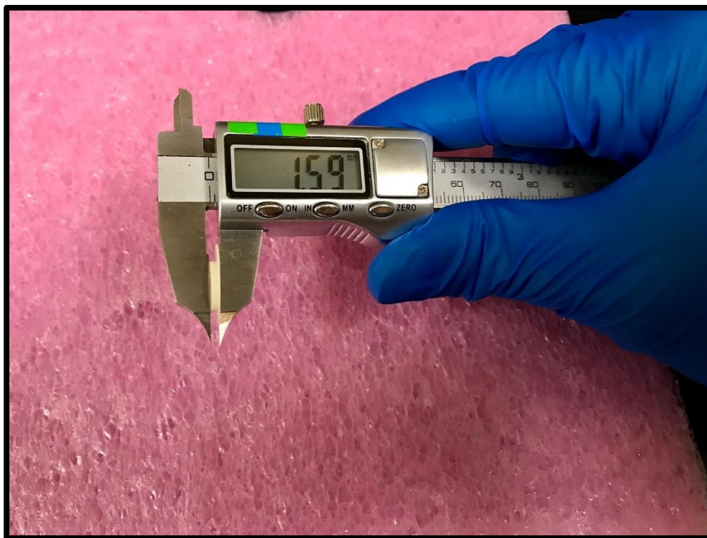
Figure 18. After each sample was cured and scanned, the sample was dislodged from the washer and measured to confirm that the thickness of the sample was between 1.3 and 1.7mm. Samples outside this thickness range were discarded and the trial was repeated.
