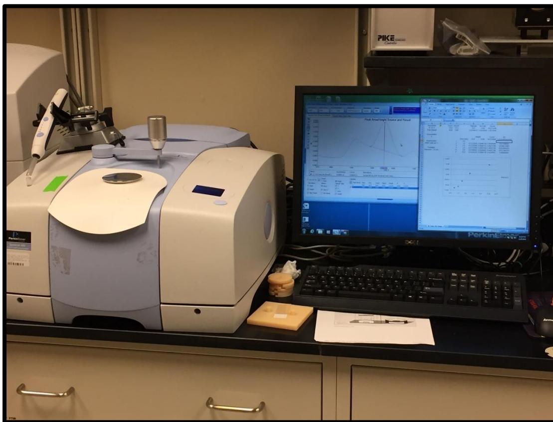
Figure 12. Fourier Transform Infrared Spectroscopy (Spectrum 400 FTIR Imaging System Perkin-Elmer, Waltham, MA) Spectrum software was utilized to capture the spectra of the sample first uncured and then one minute post cure. Each scan was captured at 2000 - 1000 \text{ cm}^{-1} wave numbers range and 6 scans per spectrum at a 8 \text{ cm}^{-1} spectral resolution.
