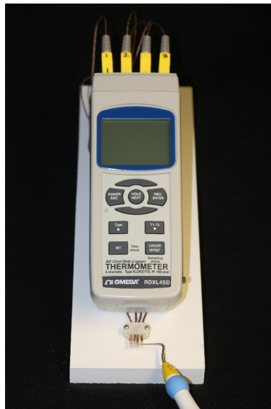
FIGURE 1: Custom 3-D printed Jig (a) schematic drawing of jig (b) Data collection setup with data logger and thermocouples placed in jig
