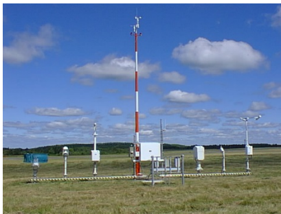
Figure 3. ASOS sensor suite, with cup-and-vane anemometer on 10 meter pole.
