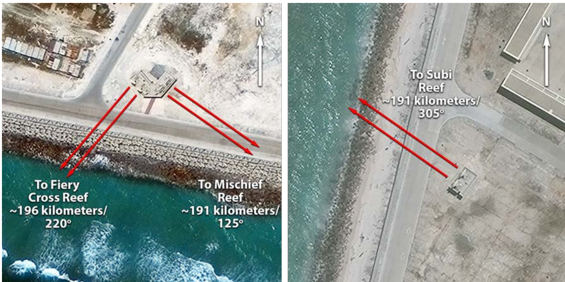
Figure 5. Subi Reef (Left) and Mischief Reef (Right) Troposcatter Terminals
