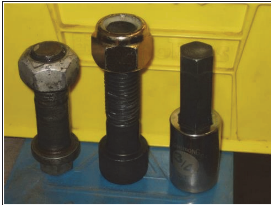
Figure 27. Non-reusable and reusable lock nuts.
