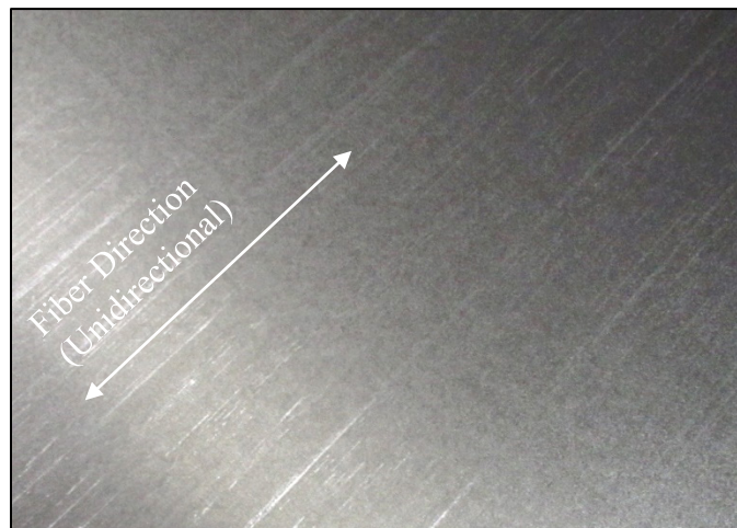
Figure 32: Uncured IM7/977-3 Preimpregnated Carbon Fiber
