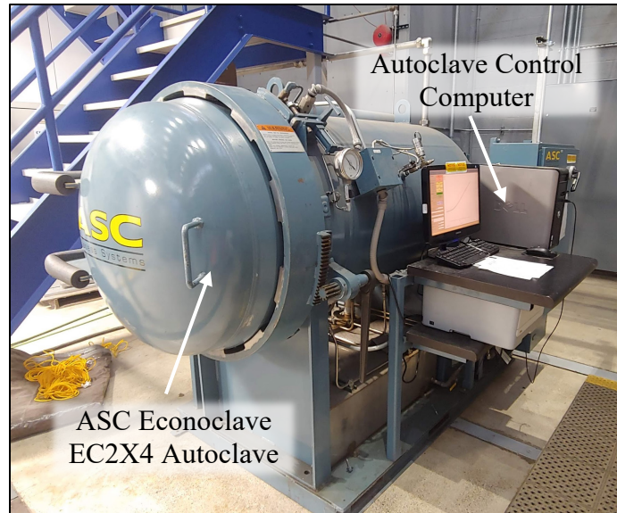
Figure 166: ASC Autoclave System
