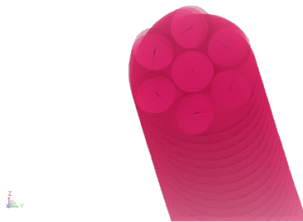
Fig. 2 End view of FEKO CAD model of a twisted power-line section
