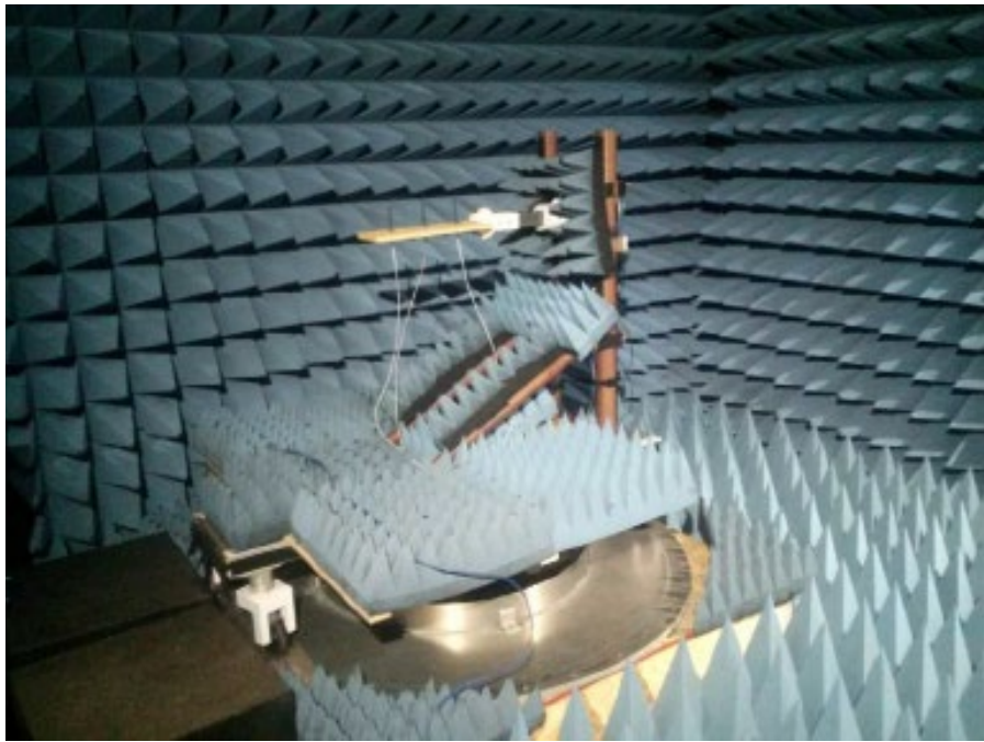
Fig. 1 GTB's antenna measurement system using a custom-designed two-stage rotation platform
