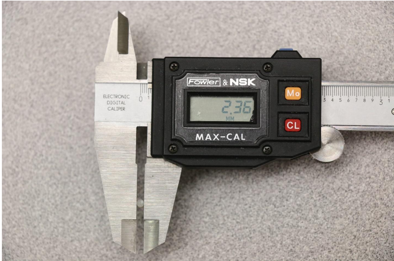
Picture 9: The diameter of each sample was measured after the shear bond strength test was finished.
