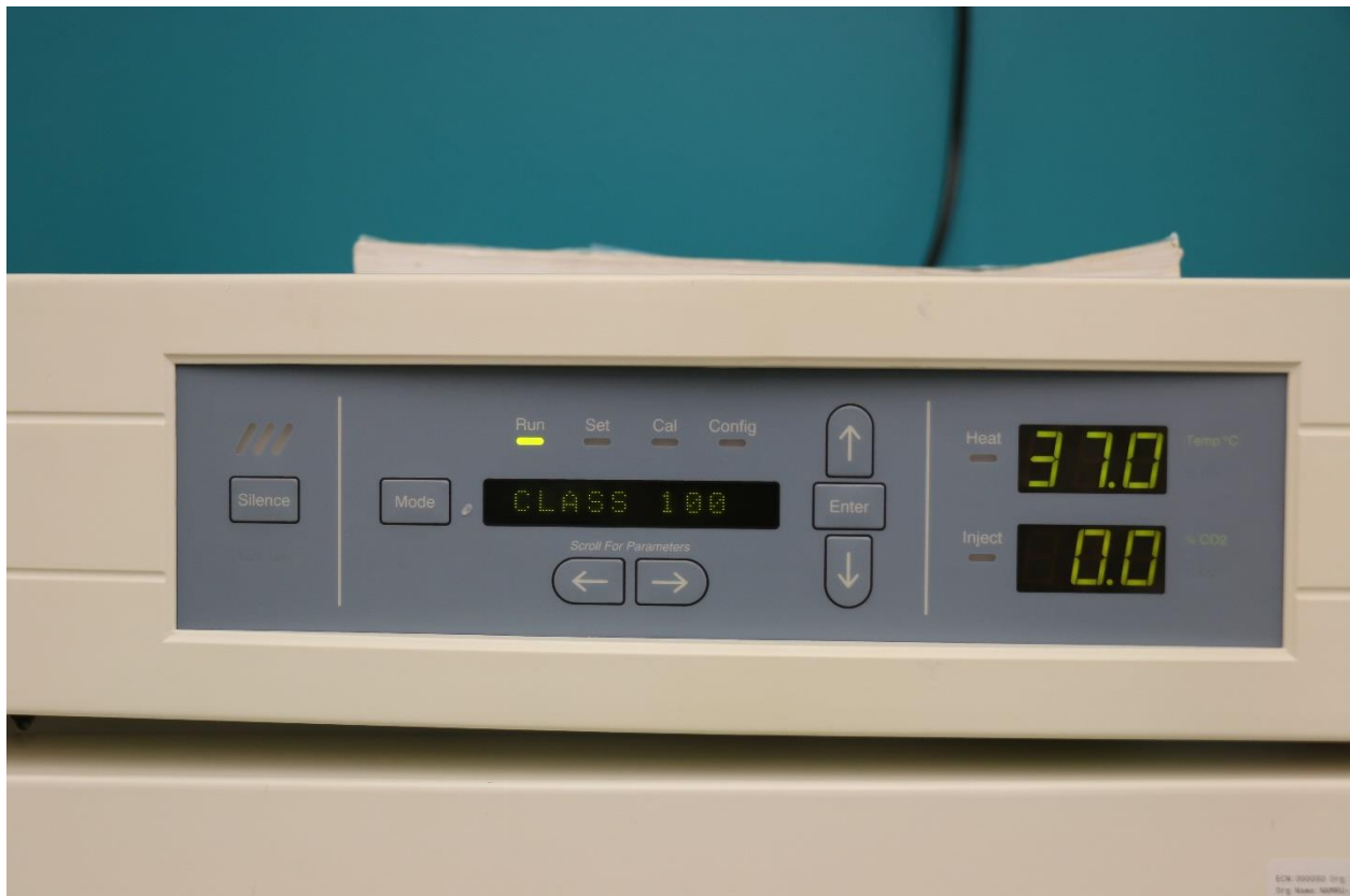
Picture 6: Samples were stored in 37°C in Thermo Forma Model 3110 Water Jacketed CO 2 Incubator for six days.
