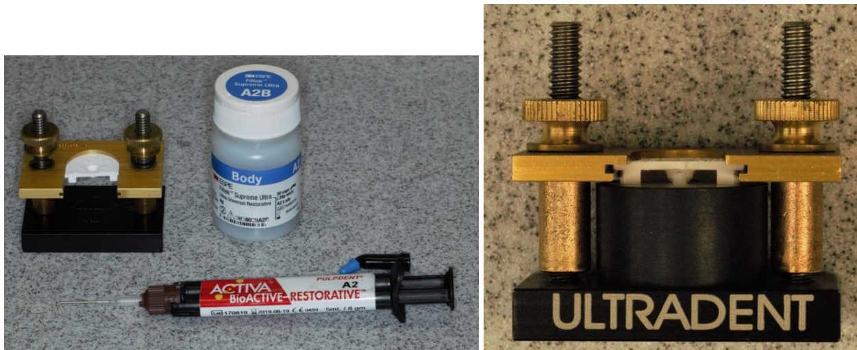
Picture 2: Initial sample preparation into black rings.
