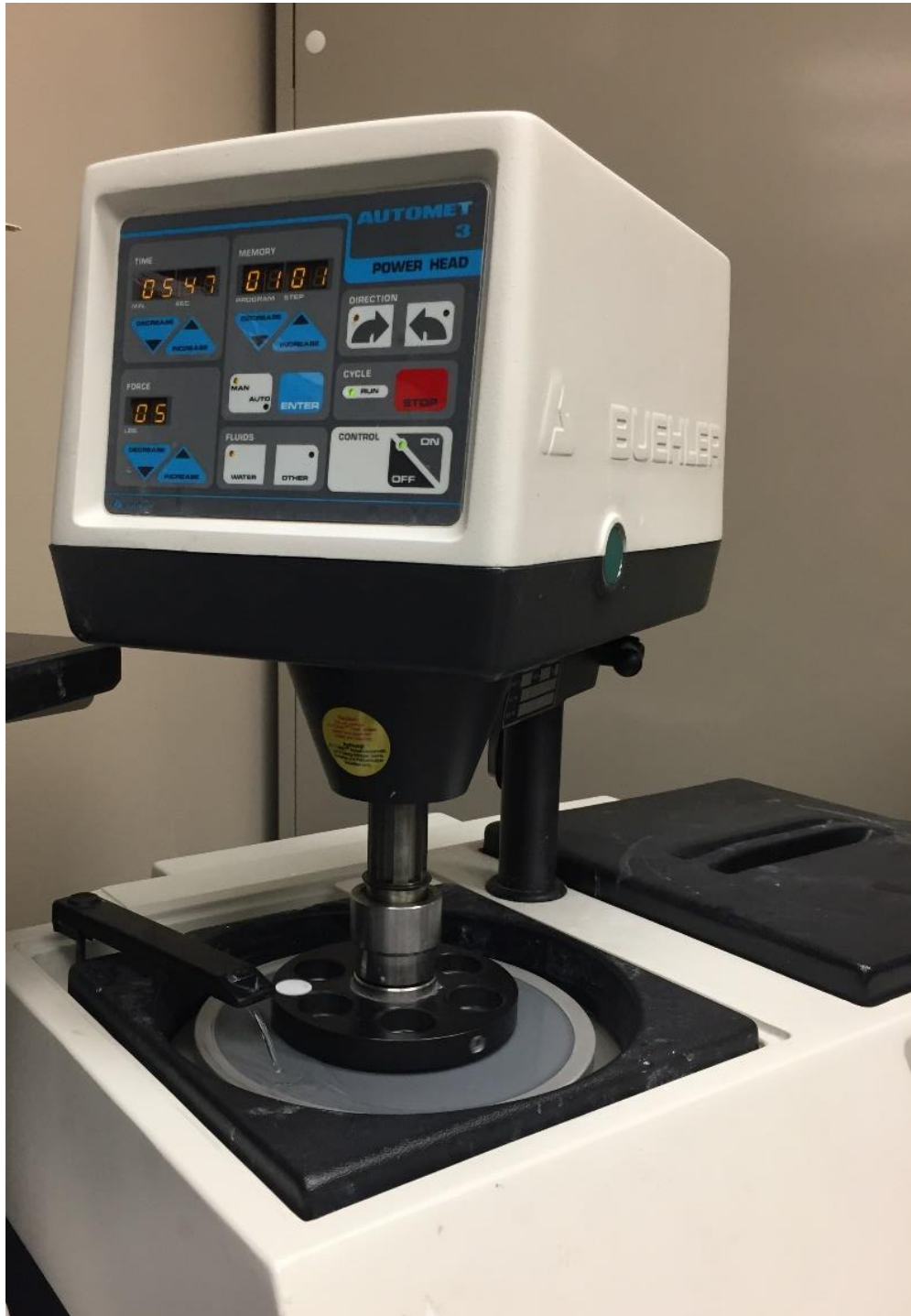
Picture 3: Six samples in the ring polished using Buehler Automet 3 Powerhead and Ecomet 6 Variable Speed Polisher.
