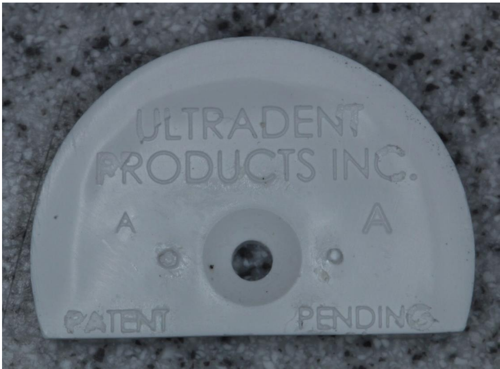
Picture 5: Standardized button mould for samples
