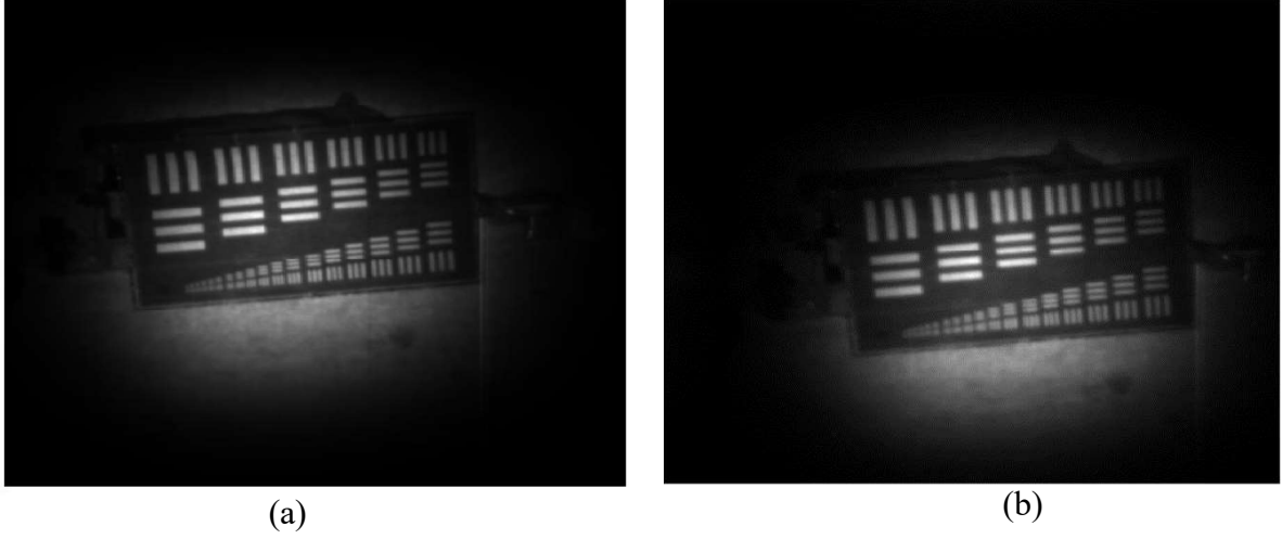
Figure 5: Beam limited target with scene shifting from frame (a) to frame (b)
