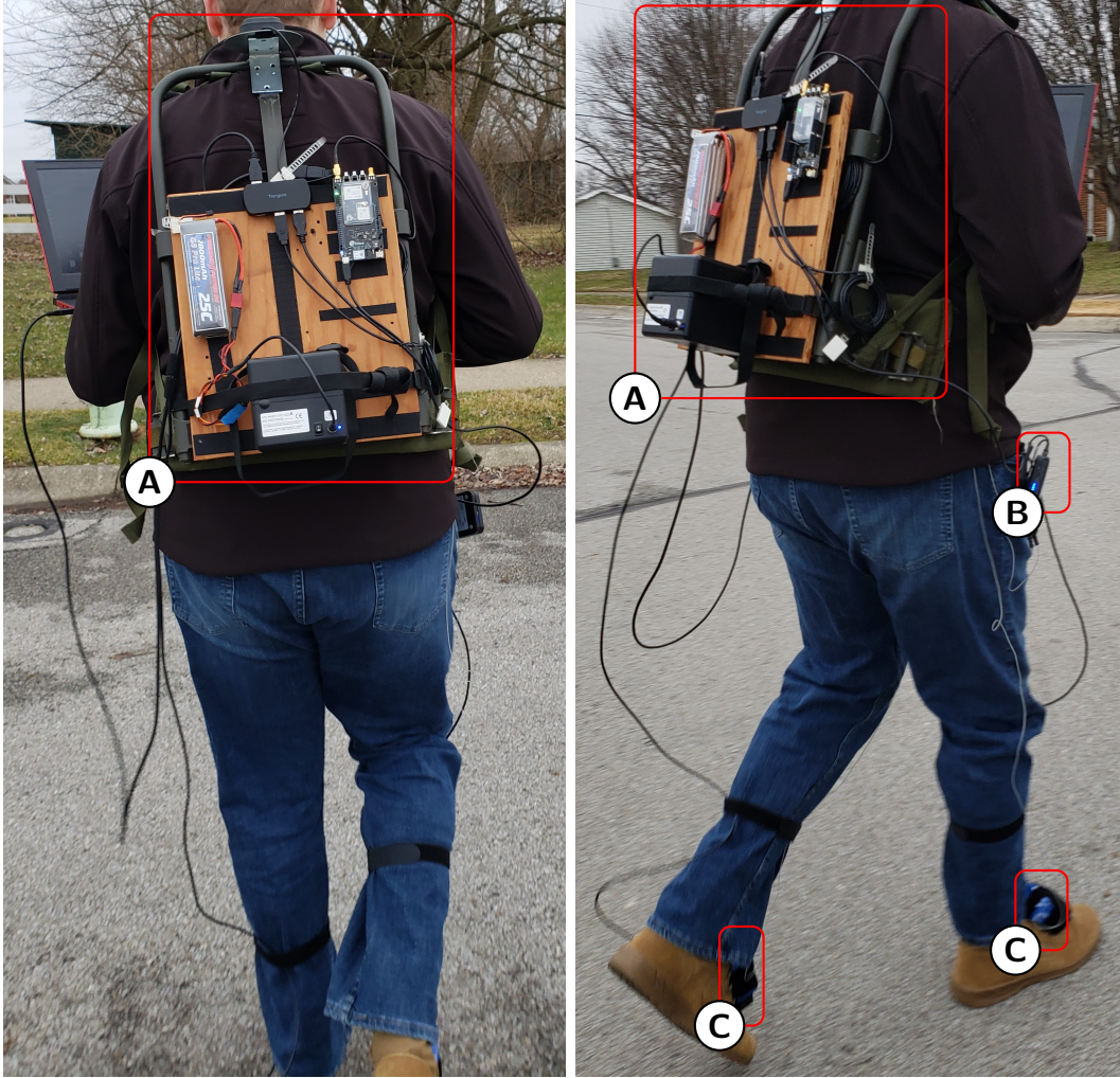
Figure 11: Left:Image of the equipment being worn with the carry pack assembly shown (A); Right: Image of the equipment being worn with the carry pack assembly(A), Polhemus system electronics unit(B) and the sensor assembly(C) visible
