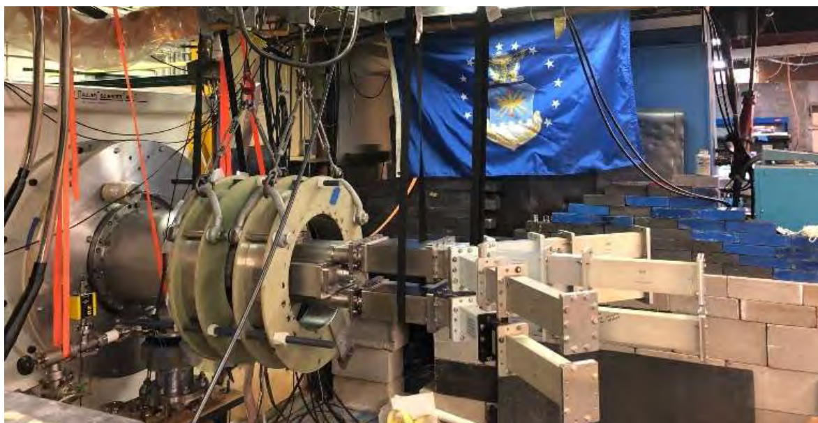
Figure 37: RPM-CACE installed on the MELBA-C driver. Six waveguide directional couplers sample each adjacent pair of the 12 RF cavities.
