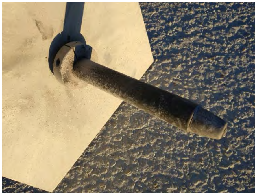
Figure 134. Shot 11: Probe 4 Shows Signs of Wear, but Is Still Useable
