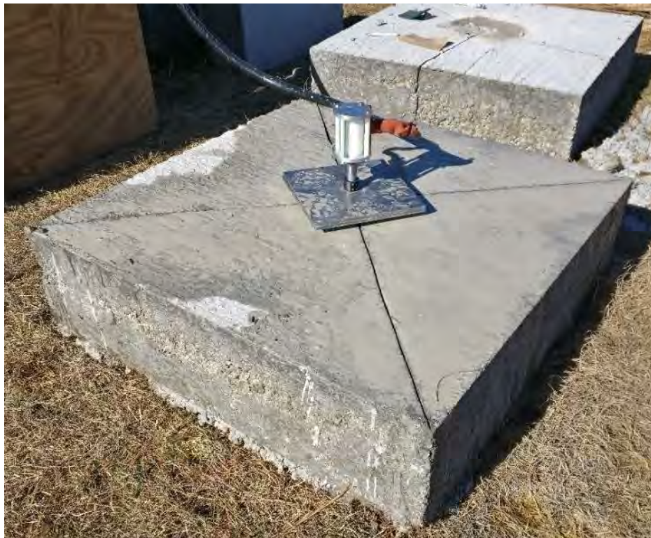
Figure 107. Shot 7: Plasma Blasting Probe Set into Concrete Test Slab 3 with 2-in-deep Pre-cuts along the Diagonals
