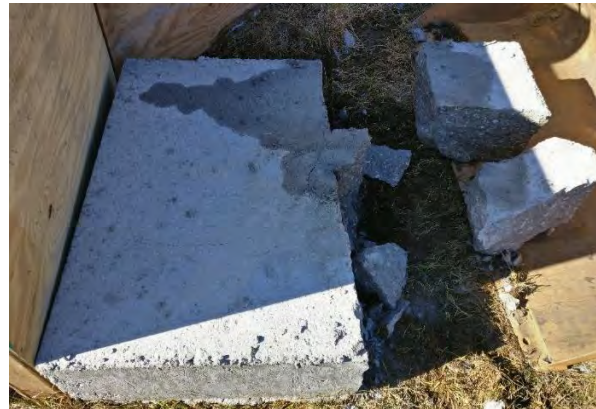
Figure 98. Shot 5: Remaining Section of Concrete Test Slab 1 after Debris Removal
