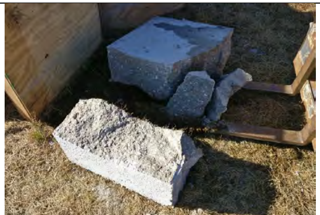
Figure 100. Remaining Pieces of Test Slab 1 Shown with Fault Line up
