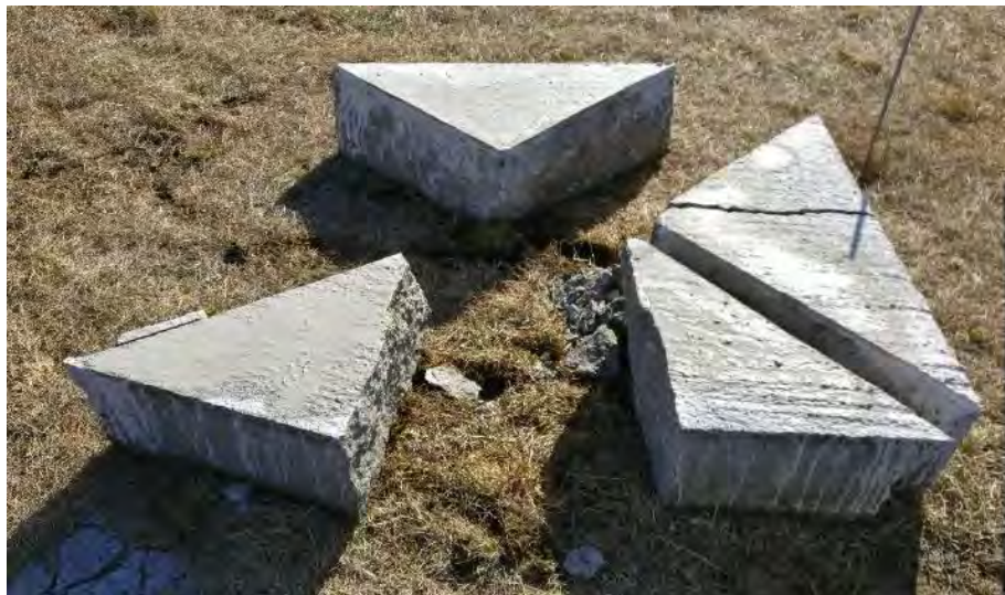
Figure 115. Shot 7: Unintended Cracks in Two Other Chunks Separated along Pre-cuts
