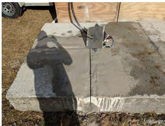
Figure 145. Shot 13: Cracked along Both Pre-cut Lines on 4 Concrete Test Slab
