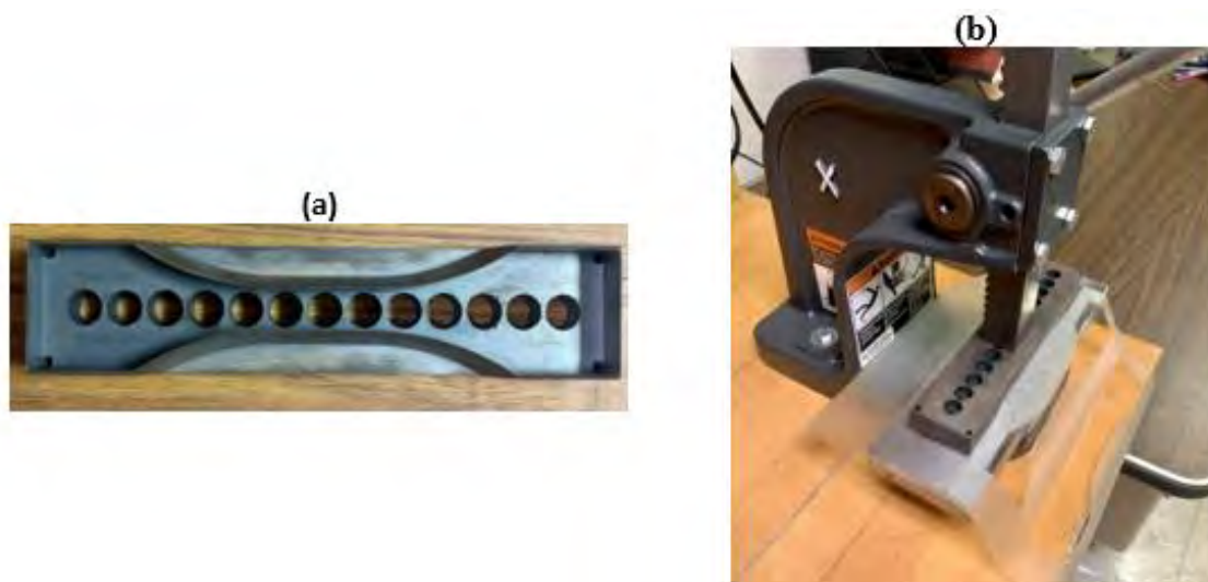
Figure 7: Drop weight specimen preparation; (a) cutting die, (b) specimen stamping.
