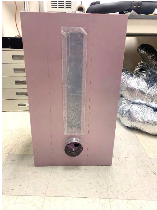
Figure 52: Temperature enclosure for drop weight testing machine.
