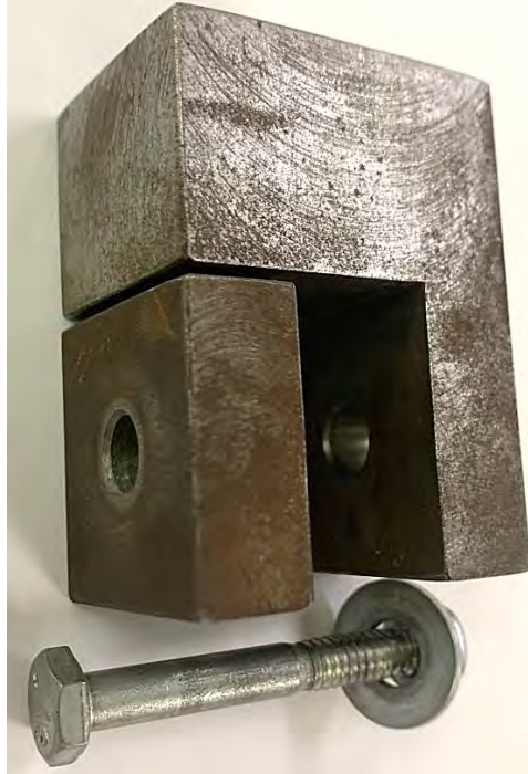
Figure 16: Upper clamp for clamping the test specimen.
