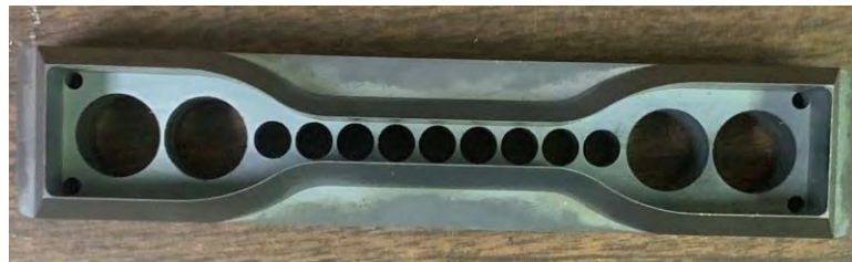
Figure 11: Quasi-static specimen cutting die.
