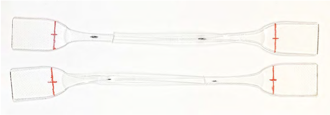
Figure 48: Failed SG quasi-static test specimens.
