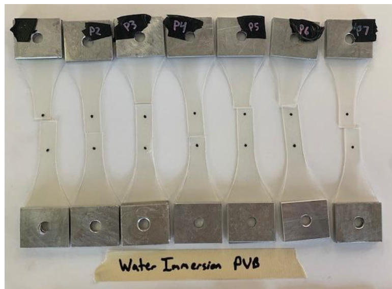
Figure 52: Immersed PVB Dynamic Specimens After Testing
