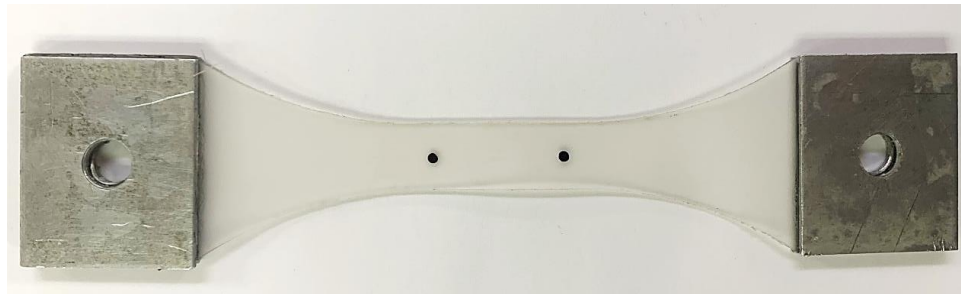
Figure 11: Dynamic Test Specimen Preparation
