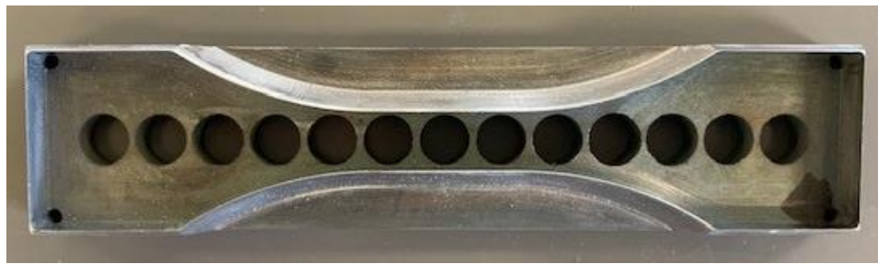
Figure 9: ASTM D638-14 Type 1 Specimen with End Tab Modifications
