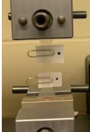
Figure 5: Paper Clip Method for EVA Specimens
