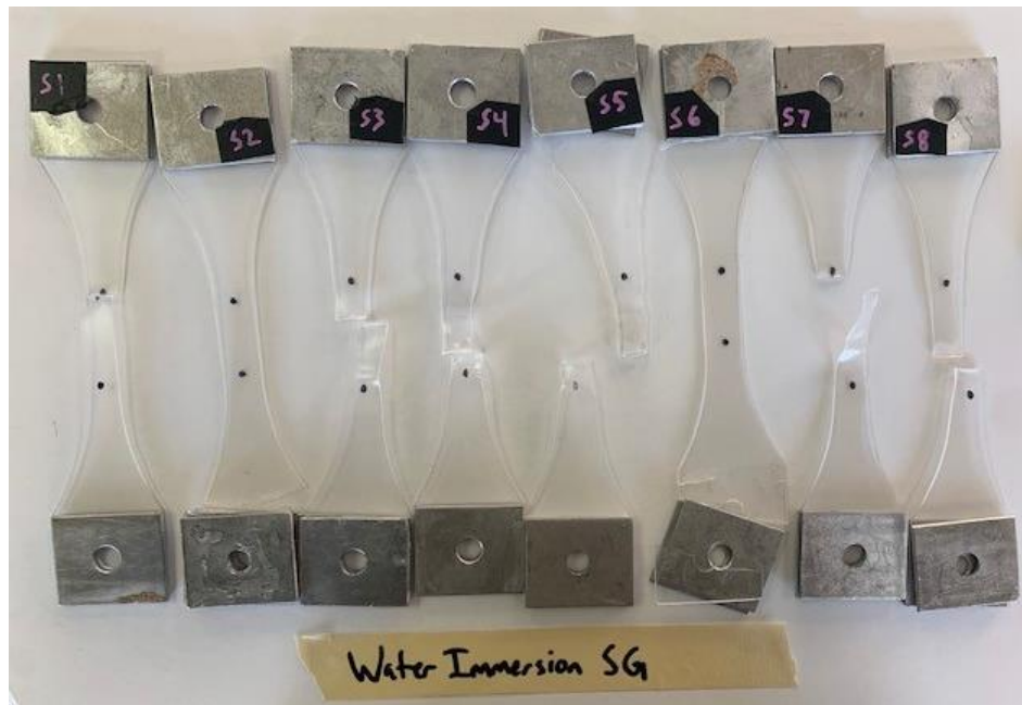
Figure 63: Immersed SG Dynamic Specimens After Testing
