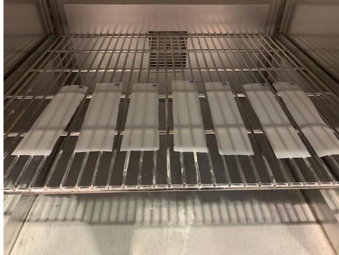
Figure 27: Oven with Dynamic PVB Specimens
