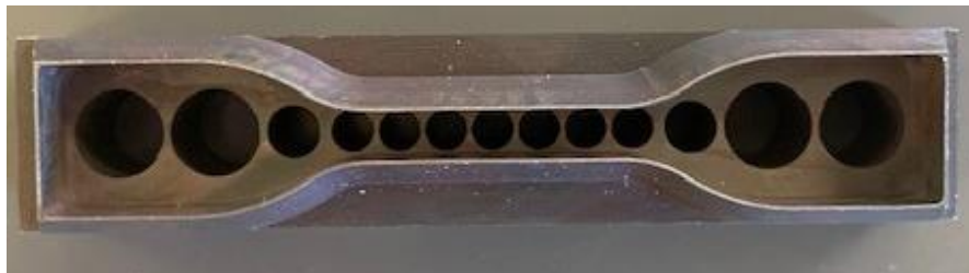
Figure 3: ASTM D638-14 Type IV Specimen Dimensions
