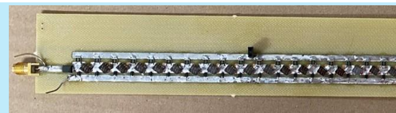
Figure 4: A 40 cell D-NLTL based on the SMV1702 model of diode. The DC bias is applied to the cathode of each diode via a 1-k \Omega surface mounted resistor.
