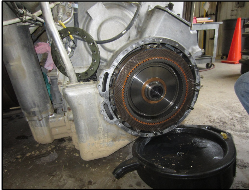
Figure E-1. Left brake pack case removed, exposing brake pack friction and steel elements (not a failure mode).
