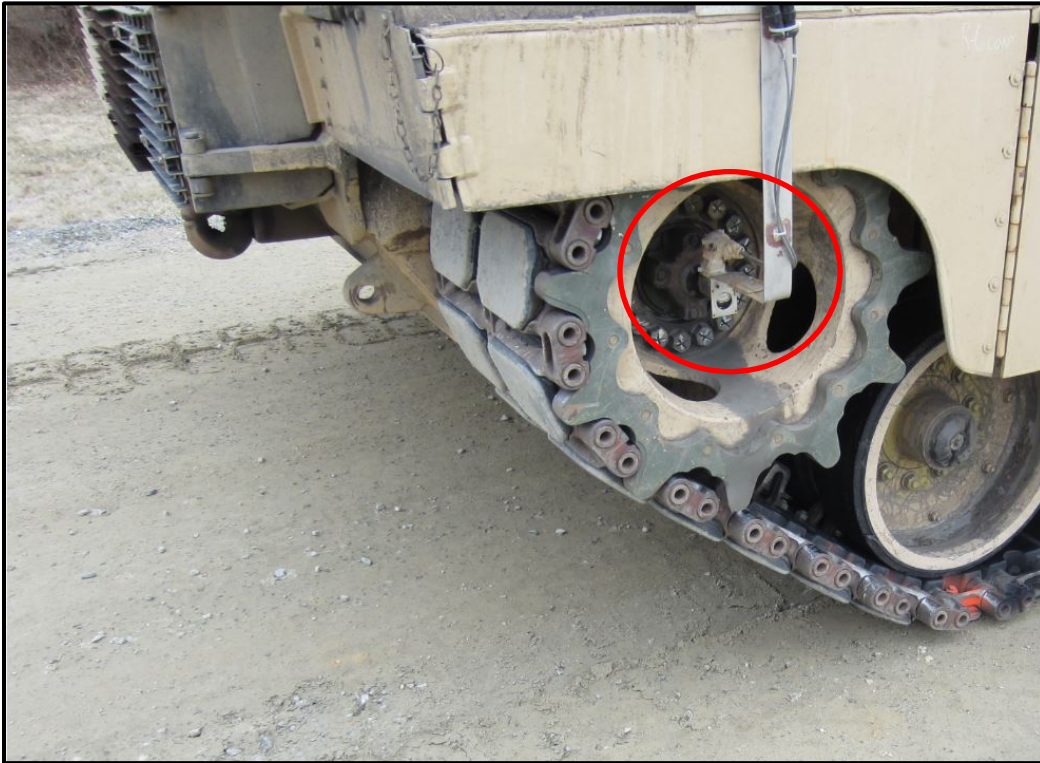
Figure A-10. Drive sprocket slip-ring and encoder used to transfer final drive torque and sprocket speed signals.
