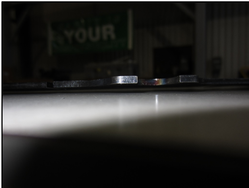
Figure E-6. Brake pack steel element coned (deformed) due to heat, side view.
