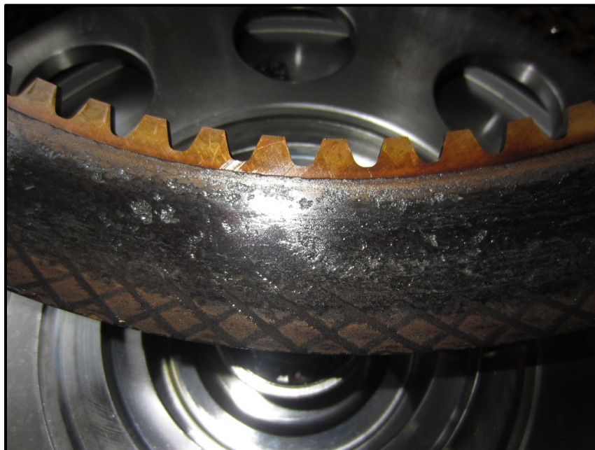
Figure E-4. Brake pack friction element lining material severely worn, disc material pitted, closer view.
