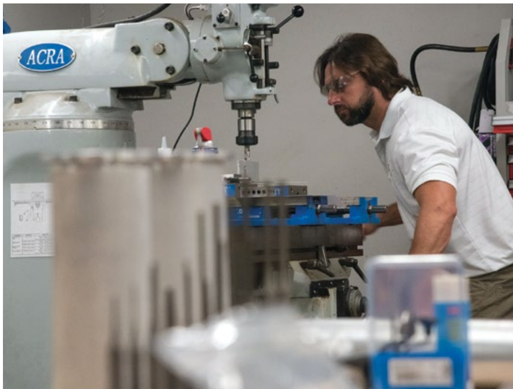
A SOFWERX technician mills a metal plate.
