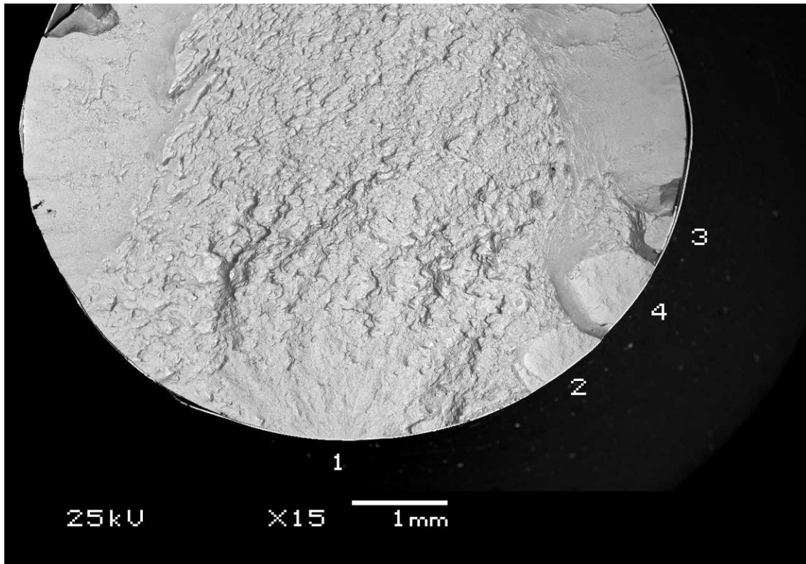
Figure A-9: SEM Fractograph of M54 Steel, Cd Coated with Ni Interlayer and Stress-Life Fatigue-Tested in Air
