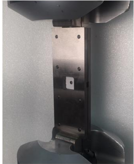
Figure A 15. Static Test Results from OHC tests, [0/90]_{2s}
