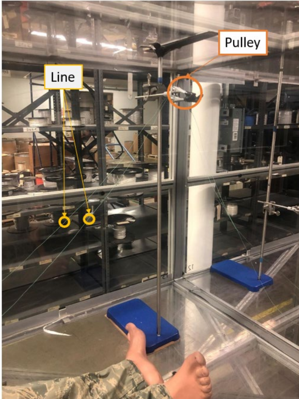
Figure 4 - Pulley system inside the chamber used for clothing removal from the mannequin.
