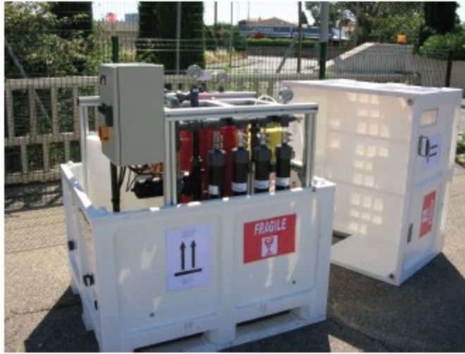
Figure 4-2: Transportable ultrafiltration system used by French firefighters (Barbot et al. 2009).
