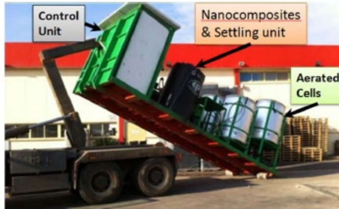
Figure 4-7: Aerated cells mobile system being placed at a winery for use (Litaor et al. 2015).
