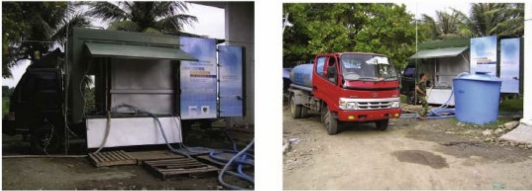
Figure 4-4: Micro hydraulic mobile water treatment plant used in Aceh, Indonesia (Garsadi et al. 2009).
