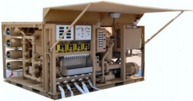
Figure 4-1: Reverse Osmosis Water Purification Unit (USAF 2011).
