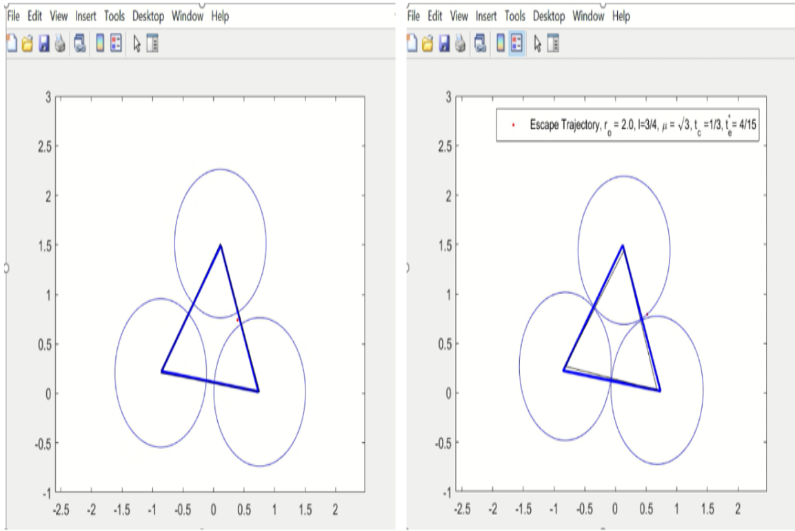
Figure 42: Equidistant pursuers: escape Trajectory, \mu = \sqrt{3} , r_o = 2.0 , l = 3/4
