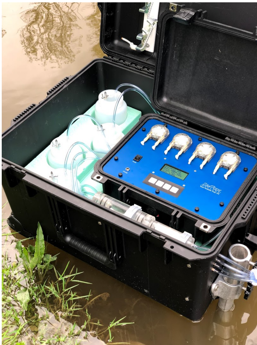
Figure D3. Pump unit, collection bottles, and iTIE units setup inside the deployment case at the Clinton River, MI, USA.
