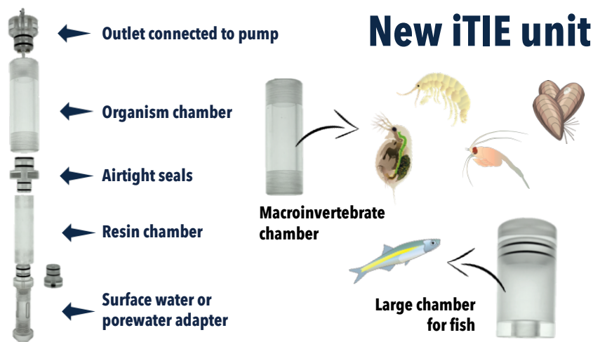
Figure 1. The current in-situ Toxicity Identification Evaluation (iTIE) fractionation system – Prototype 3
