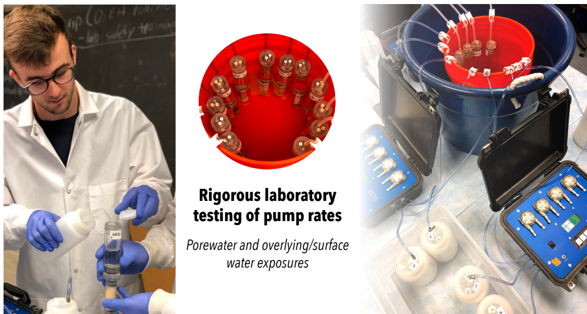
Figure 3. Laboratory testing of pump rates and resin selection for different contaminants of concern.
