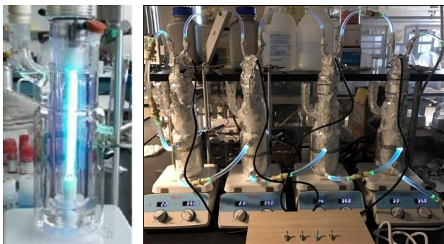
Figure E1. The UV reactors at UC Riverside.
