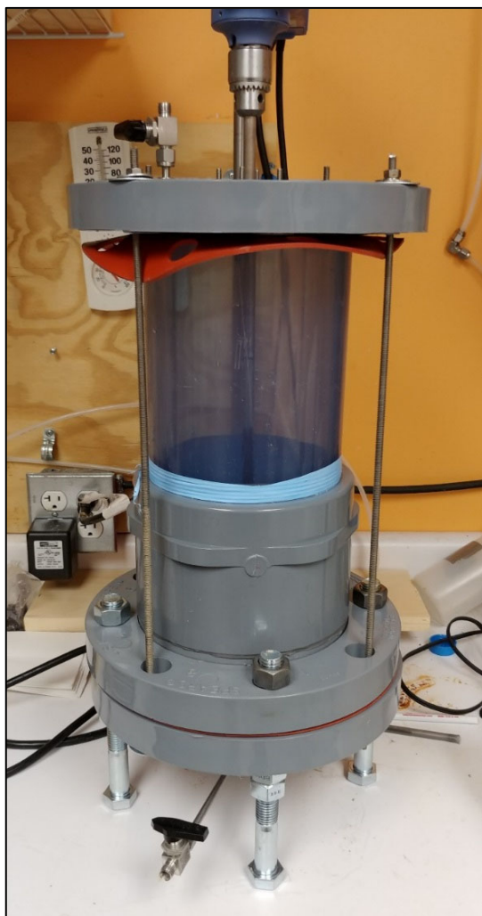
Figure 3: The sand/silt/clay IDW soil fraction was treated inside a 5 liter clear PVC slurry reactor.
