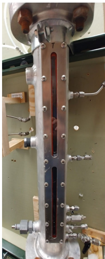
Figure 5: Pilot-scale UV-irradiation reactor.
