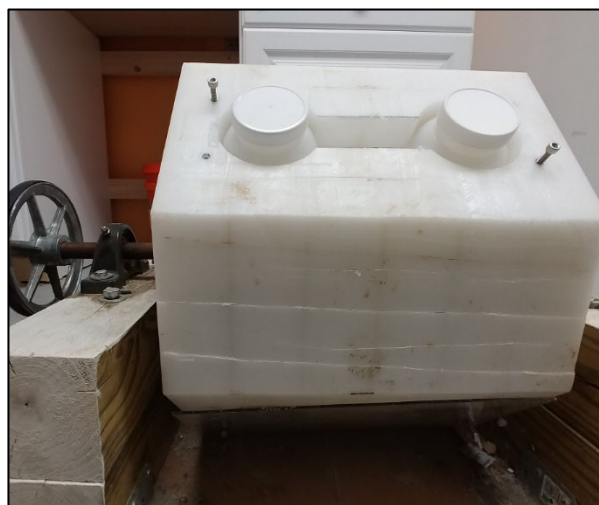
Figure 2: Tumbler for rinsing coarser IDW soil.
