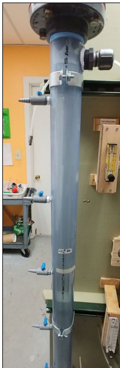
Figure 4: A batch-scale foam fractionation reactor was build using plastic column material. The dimensions of the system were 3" diameter and 6' long
