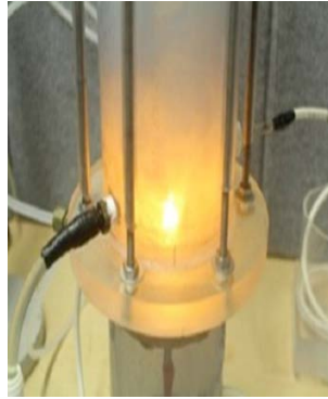
Figure 2. 2. Photograph (left) and schematic (right) of gliding arc plasma system with plasmatron submerged into liquid solution.
