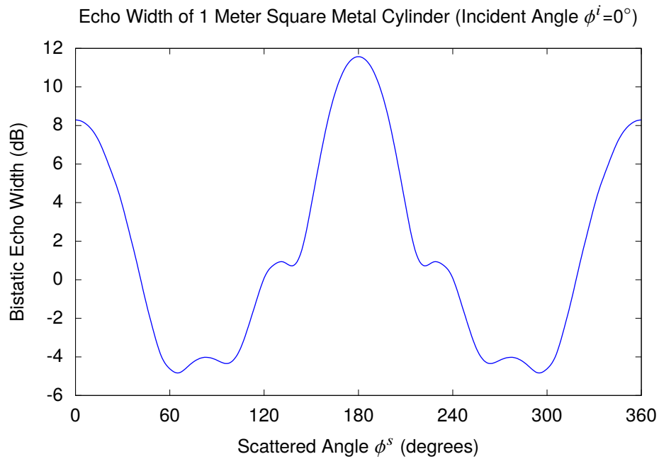
Fig. 5—Bistatic echo width of a 1 meter metal square cylinder at 300 MHz for a Yee FDTD grid with \Delta x = 0.05 meters, 800 time steps, a 16-cell cosine PML, 4 cells between the PML and integration surface, and 3 cells between the integration surface and the TF/SF boundary.
