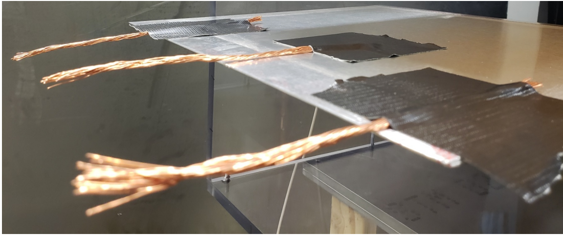
Figure 17. Airfoil with three copper wicks attached to the tapered edge with an inter-wick spacing of 7.62 cm. All wicks extend 7.62 cm past the edge.
