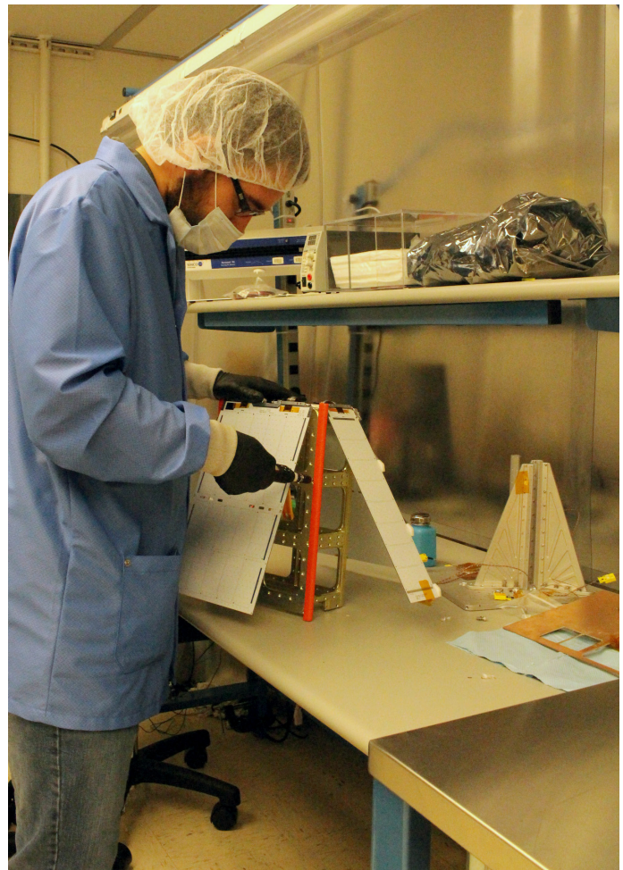
A research assistant from the Center for Space Research and Assurance assembles a Grissom satellite chassis in the CSRA’s clean room. CSRA students learn Space Vehicle Design by integrating the chassis with a research payload, subjecting it to vibration and thermal-vacuum tests to predict whether it will survive the harsh environment during launch and on orbit. (Air Force photo)
