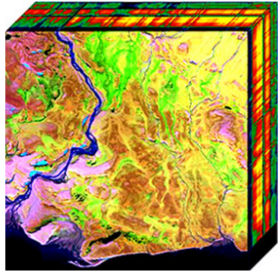
Figure 1: Data cube of hyperspectral imagery. Each slice images the intensity of light in a fixed wavelength. One may discern the chemical composition of a pixel (e.g. water, foliage, rock) from how the light intensity varies with wavelength. (From N. M. Short, Two-dimensional projection of a hyperspectral cube, 2013.)
