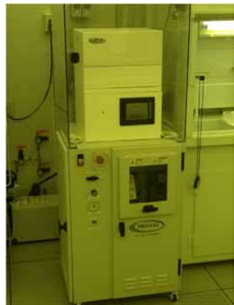
Figure 2: HF vapor etching system for etching silicon dioxide without damaging metal contacts as well as enabling high-aspect MEMS and NEMS releases – only 4 in the USA.
