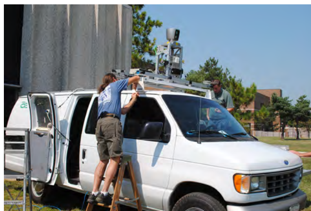
ANT Center Navigation Sensor Rack being mounted on Ohio University's Test Van for ASPN Data Collection.
