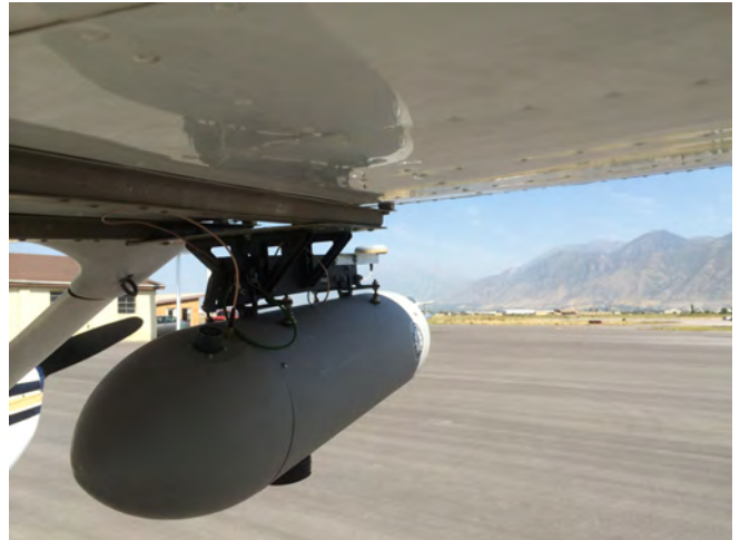
UVAN pod mounted to right wing of Cessna 172
