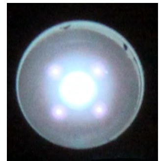
Right: 20 Watt Micro-Hall effect thruster operating with xenon propellant.
