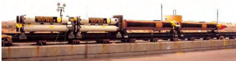
Figure 2. The setup at Holloman Experimental Test Track consisted of 4 rocket powered sleds. AFIT’s research methodology was instrumental in assisting Holloman AFB to achieve the world land speed record of Mach 8.5 for the rocket sled.
