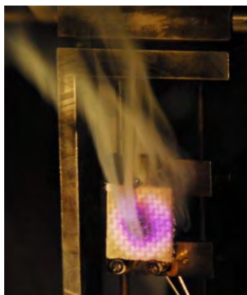
Figure 1. Solid state laser irradiation of fiberglass.
