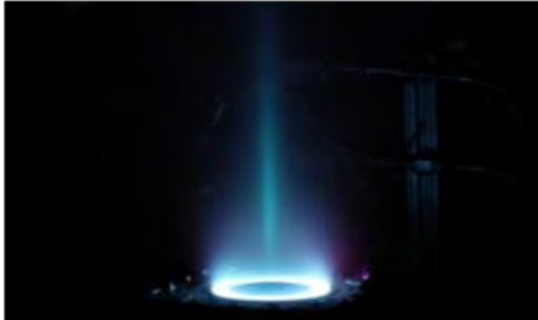
1500 Watt Hall effect thruster operating with xenon propellant at the SPASS Laboratory.
