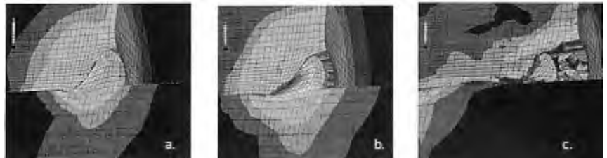
Figure 1. Time sequence of wear development using AFIT’s 3D FE high velocity wear model of the collision of a slipper (upper object) with an asperity on a rail (lower object).
