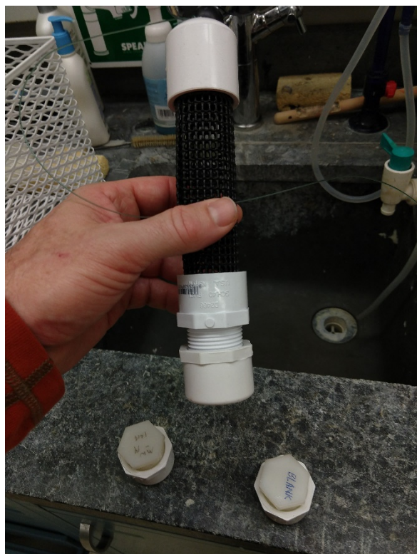
Figure 11. NaOH Trap Showing Support and Reservoir
