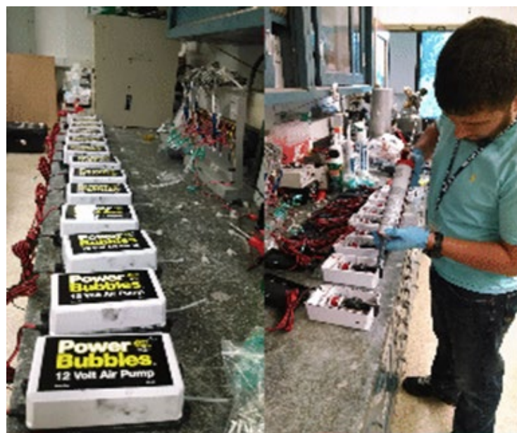
Figure 8. Well Headspace Gas Recirculating Pumps, Sealed
