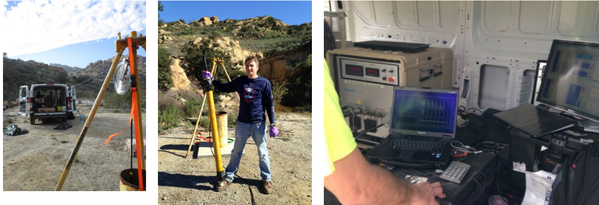
Figure 6. 28: a) Photo showing SSFL borehole C4 with mobile logging system in the distance, b) NMR tool used for measuring water content in the formation surrounding the borehole, and c) NMR control unit and computer for viewing measurements and processing data for water-content, pore-size distribution, and hydraulic conductivity estimates. The NMR logging system used for this investigation is lightweight and mobile relative to conventional NMR systems used in the oil industry.
