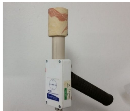
Figure 6. 13: Bartington MS2K sensor measuring MS on a HC core.
