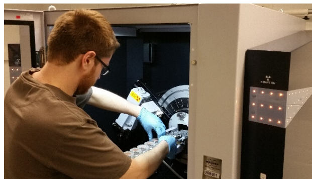
Figure 6. 7: A sample loaded into Bruker D8 Advance used for XRD measurements.
