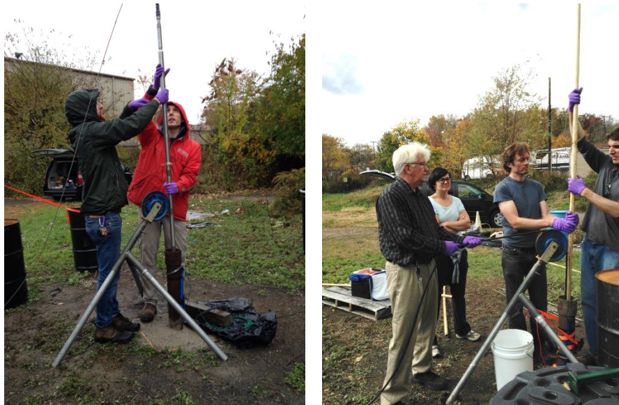
Figure 6. 25: a) Collection of standard logs in NAWC 94-BR – photo showing the lowering of the full-wave form sonic tool into the borehole and b) Collection of NMR in 94-BR – photo showing the NMR tool with fixed magnets being pushed through the steel casing into the open section of the borehole.
