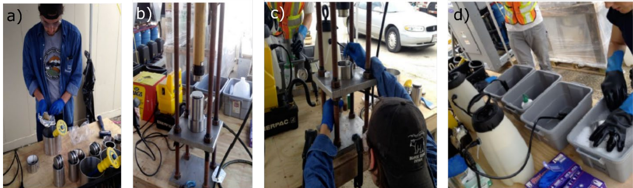
Figure 6. 4: VOC sample processing in the field: a) Trimming the core rind exposed to drilling fluids, b) crushing the sample using a hydraulic press and stainless steel crushing cells in a setup designed to minimize exposure time to air, c) sample transfer to pre-preserved (MeOH) vials, and d) 5 step process for decontamination of core crushing equipment applied between samples.
