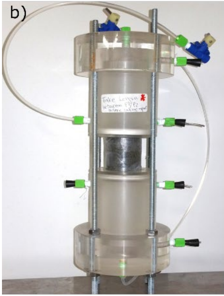
Figure 6. 16: a) Schematic of CR sample holder used for data collection. A geometric factor correction was necessary to account for the geometry of the sample holder b) Sample setup within a sample holder c) CR data collection in environmental chamber.
