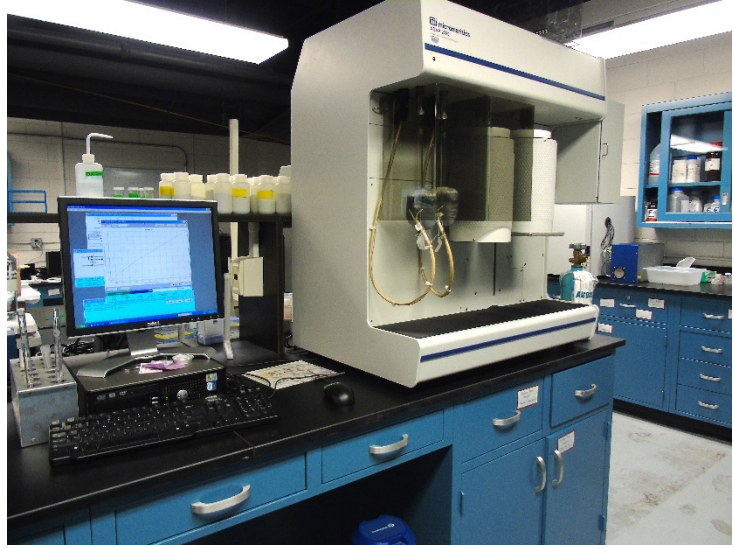
Figure 6. 11: On-going BET data collection. Shown are two samples in the degas port and one sample where BET data are being collected.
