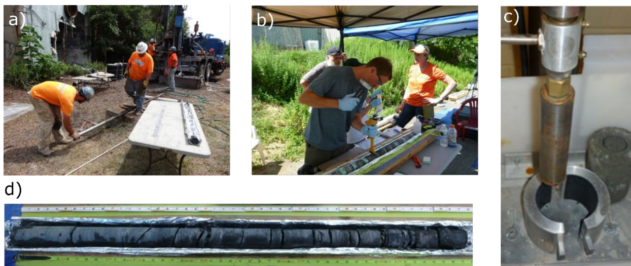
Figure 6. 3: a) HQ triple tube rock coring at the NAWC site (corehole 94BR), b) field rock core subsampling, c) laboratory subcoring of rock core samples, and d) example of extracted core from borehole before field subsampling.
