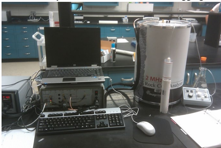
Figure 6. 14: RoCA instrument used to collect all NMR data.
