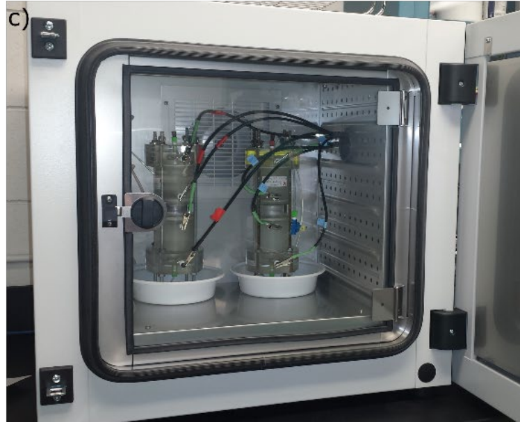
Figure 6. 16: a) Schematic of CR sample holder used for data collection. A geometric factor correction was necessary to account for the geometry of the sample holder b) Sample setup within a sample holder c) CR data collection in environmental chamber.
