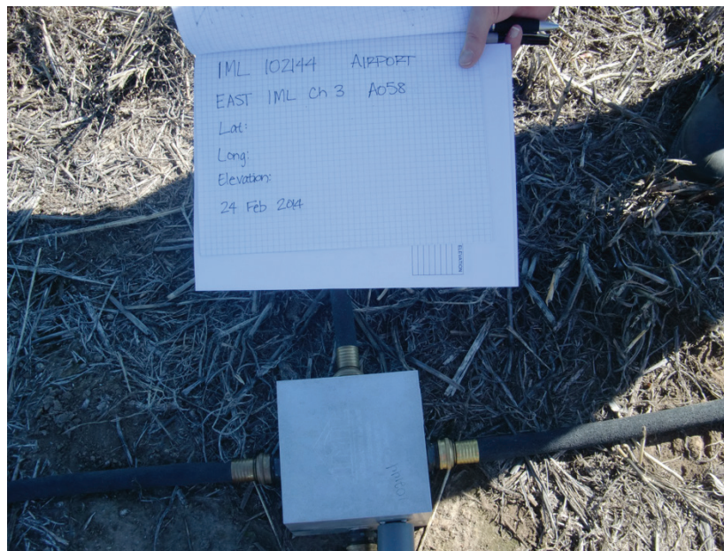
Figure 7. Example of an IML sensor with four porous hoses.
