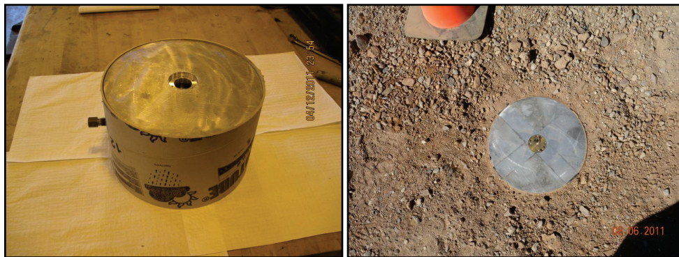
Figure 4. Pressure transducer mount (left) and installed mount (right).
