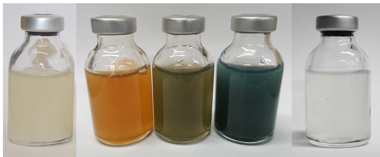
Figure S5: Reactors of differently prepared low Fe content clay mineral SWy-2: native, amended with aqueous Fe(II) at concentrations of 1.9 mM, 4.9 mM, or 20.1 mM, and dithionite-reduced (from left to right).
