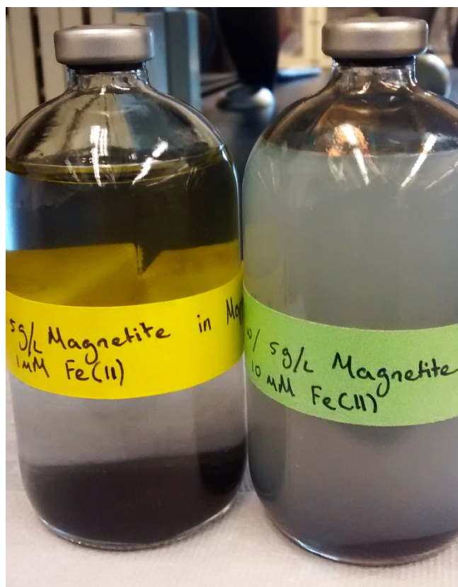
Figure S1. Photographs of reactors containing 5 g/L magnetite reacted with low Fe(II) ( \sim 1 mM, left) and high Fe(II) ( \sim 10 mM, right). The solids on the right contain white \text{Fe}(\text{OH})_2(\text{s}) . Conditions: 10 mM MOPs buffer at pH 8.0, and 50 \mu\text{M} TCE.
