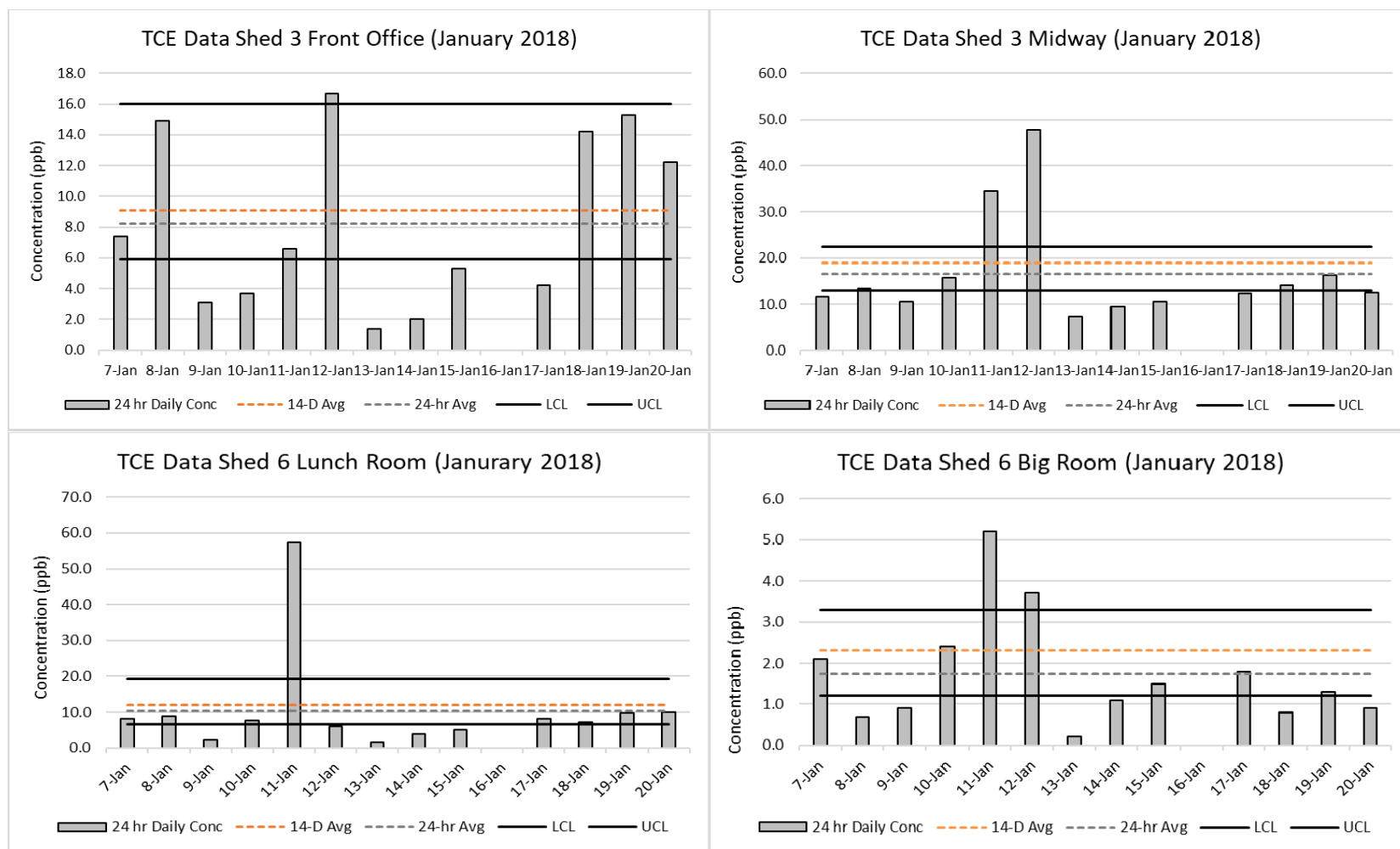
Figure 14. Comparative Analysis of Traditional Diaphragm Daily Samples and Capillary Controller 14-day Samples in Four Locations During a 2-week Period in January, 2018.
