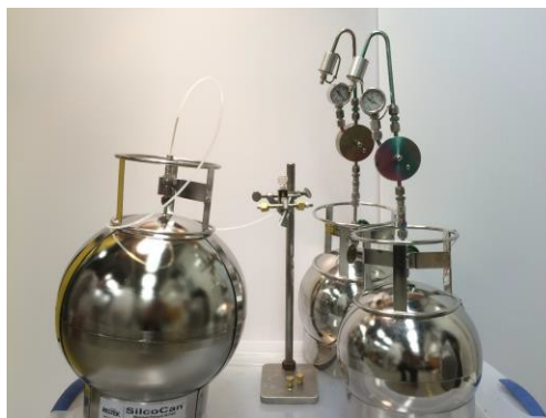
Figure 7. Typical Monitoring Station at Each Location with the Additional 1 Quality Control 24-h Canister.
