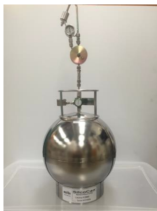
Figure 9. Silco Coated CS1200ES Flow Controller Attached to a 6-L Silco Canister.
