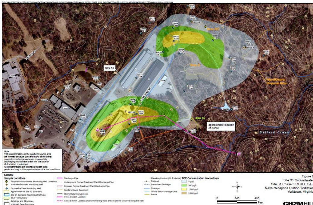
Figure 6. TCE Groundwater Plume as of 2014.
