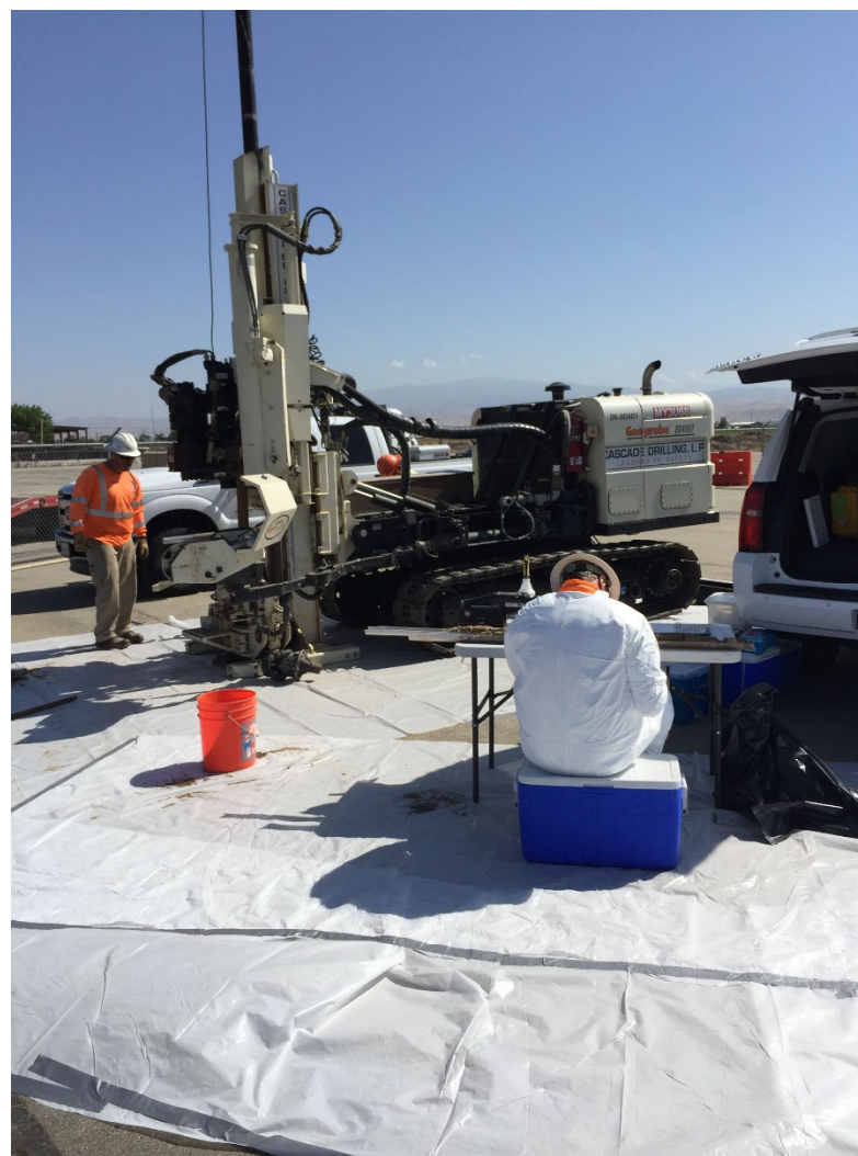
Photo 2 APTIM geologist logging soil cores.
