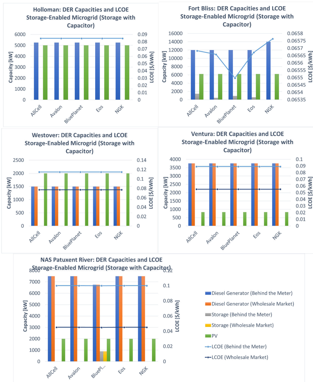
Figure ES-2a. Optimal Microgrid Portfolio and Levelized Cost of Electricity of Each Base Modeled for Each Battery Technology Paired with a Ultracapacitor/UPS System that Can Extend the Expected Life with No ITC or MACRS Incentives
