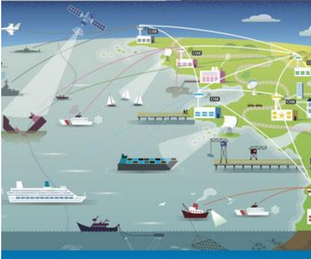
Figure 15. VTS concept. Example schematic of a VTS port area, illustrating the diverse range of vessel traffic and various surveilled and non-surveilled systems used to create a port's "traffic image." 9
