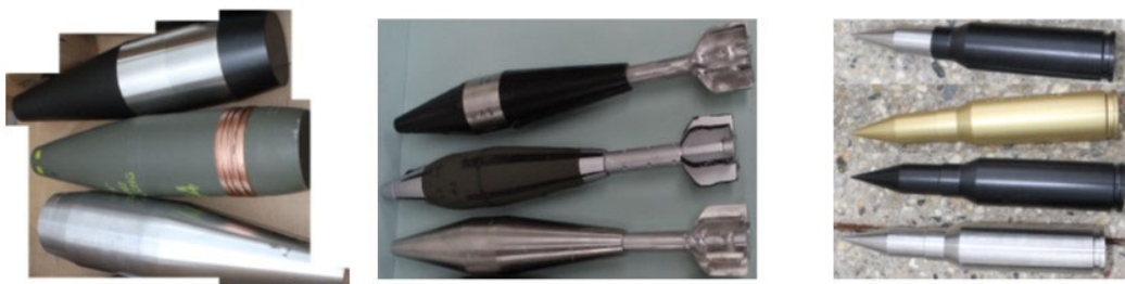
Figure 1. Four types of fabricated surrogate, purchased replica, and fabricated replica of (left) 155 mm HE M107, (middle) 81 mm mortar, and (right) 25mm and 20 mm cartridges (from Calantoni et al. 2014).
