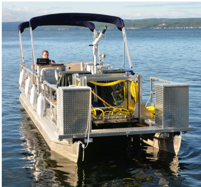
Figure 4: The Sound Hunter test platform is a nine-meter pontoon boat. The projector and receive array are shown here mounted in the forward portion of the boat. These components are mounted in a rectangular frame that is lowered into the water during testing.
