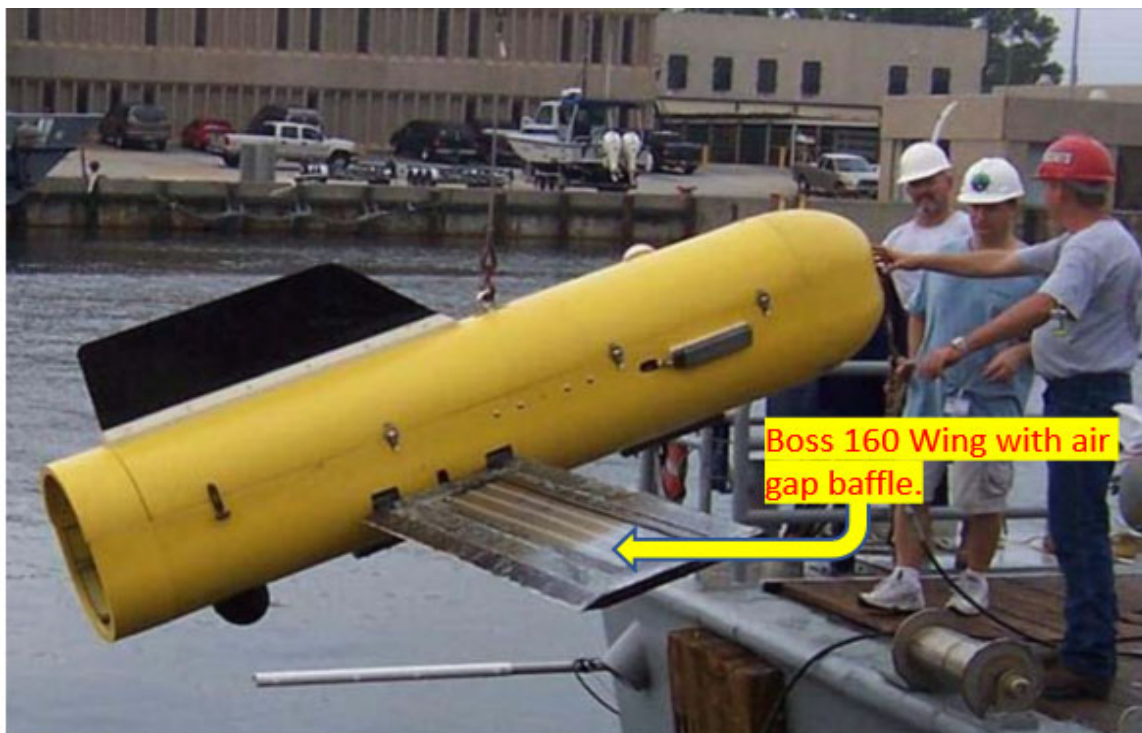
Figure 49. SERDP BOSS-160 demonstrator being deployed in Panama City, FL. Each carbon fiber wing is embedded with 4 rows by 20 hydrophone staves with a 2" pitch. The optionally floodable air gap baffle is seen at the wing tops.
