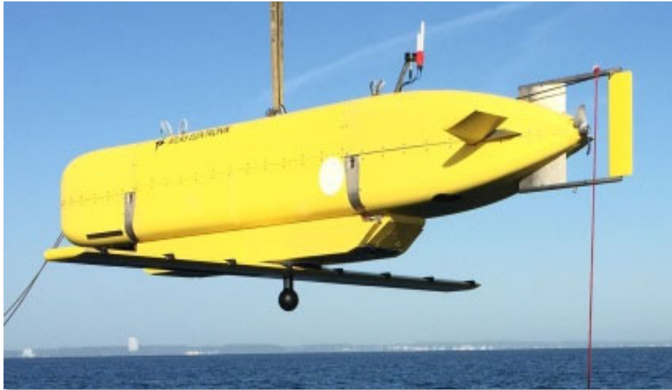
Figure 47. Atlas Sea Horse with eBOSS Payload. Hydrophone wing consists of 4 panels, 64 channels total, with 2" spacing between segments. The wing rotates into the across-track position after deployment.
