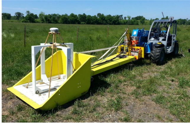
Figure 1. Left : MetalMapper sensor geometry. Red dashed lines indicate the three transmitter coils and solid black lines are the 7 3-component, receiver cubes. Right : MetalMapper setup for cued collection at SWPG. Image from “ Technical Report: ESTCP Munitions Response Live Site Demonstrations – Former Southwestern Proving Ground, Arkansas, ESTCP Project MR-201231. ” (Steigerwalt, 2015).
