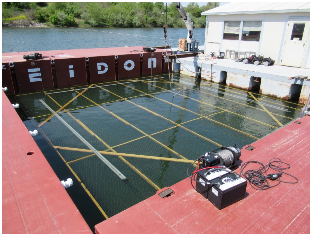
Figure 3. Catch Net and Electric Hoists
