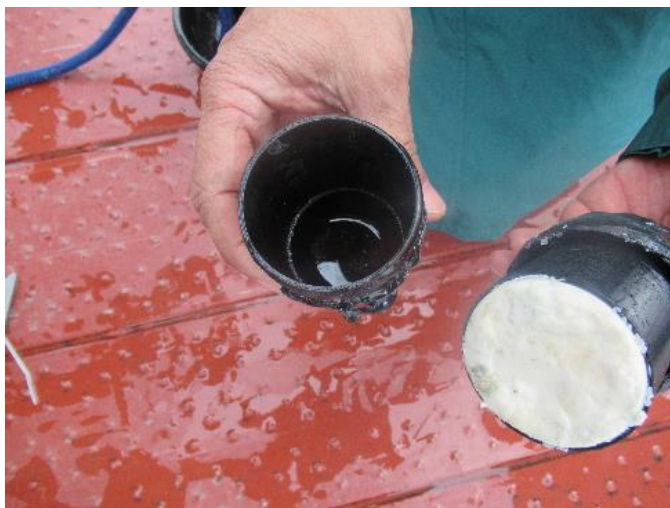
Figure 18. Water Inside EGP Device after Submersion
