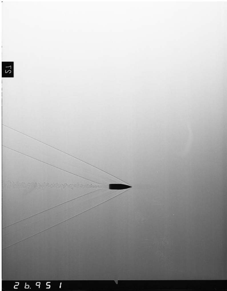
Fig. 3 Sample shadowgraph on Mylar-backed film
